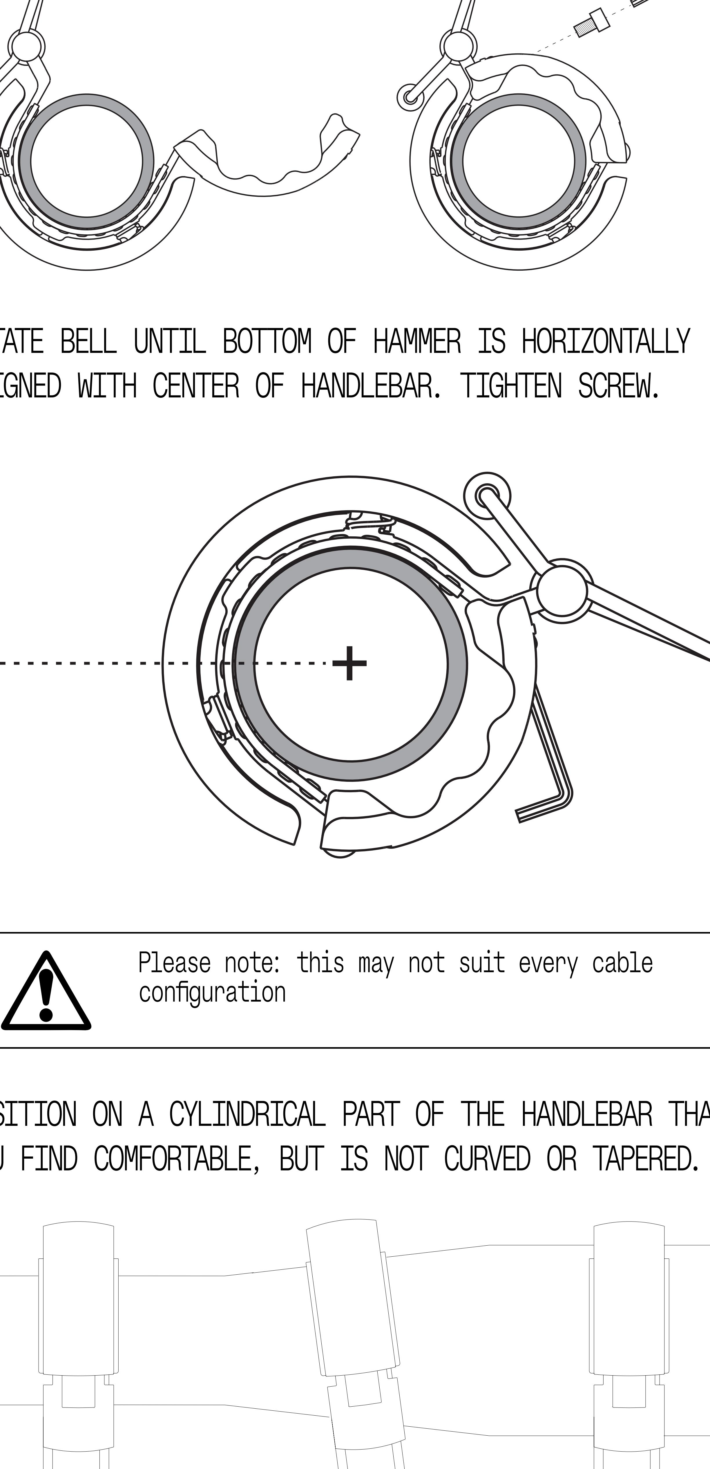
ASSEMBLE BELL ON HANDLEBAR UPSIDE DOWN. INSERT SCREW, BUT DO NOT TIGHTEN.
